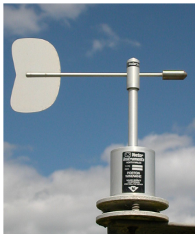
A windvane used for measuring wind direction.
