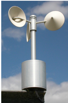
A cup anemometer used for measuring wind speed.
